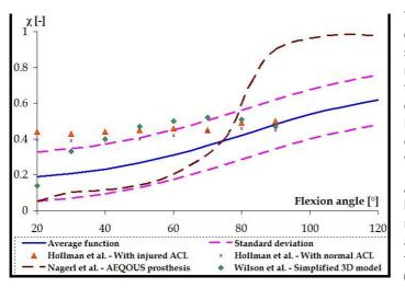
The ratio has been determined by means of a complex multi-body system, built and simulated, by the MSC.ADAMS. The slide-roll ratio curves has been introduced in the active functional arc of the knee in case of several commercial- and one prototype prostheses. By these curves it becomes possible to estimate the applicable sliding-rolling ratio with respect to the flexion angle.
