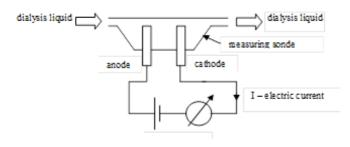
Taking into account that the estimation of the composed uncertainty is not very simple in the specific conditions regarding the working practice of the dialysis, a simplified uncertainty estimation for the conductivity measurement will be proposed. The measurement principle of the conductivity consist in an electrical circuit composed from
